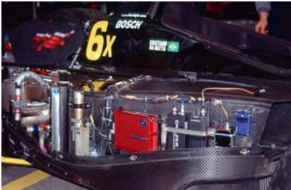
A data-acquisition processor (red box) mounted in a CART car.
