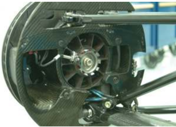
Feedback from an inductive sensor and toothed reluctor ring mounted on each wheel hub accurately measure wheel speed. An onboard computer uses this information to calculate tire slip.
